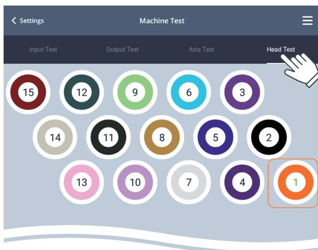
It is mainly used for detecting whether thread break sensor on the head is normal.
