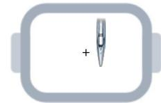
3. Use direction key to move the hoop until the hoop center point is overlapped with the lower needle position of current stitch (use reset key to observe the stitch hole); the display value is X/Y center point value, click save to finish.
