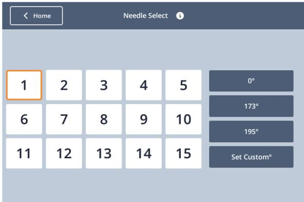
1. The left [Numeric key] is the target needle bar number. Click the number to change to the designated needle bar.
