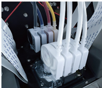
Arrangement of nozzle ink inlet: K C M Y W W W W
