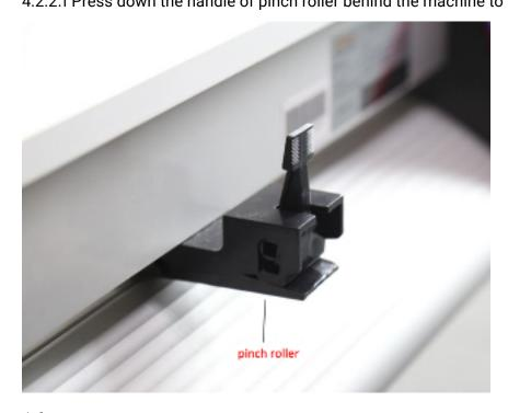
4.2.2.2 Insert the media into the space between the pinch roller and grit roller, and pull out media to the appropriate length at the front.
