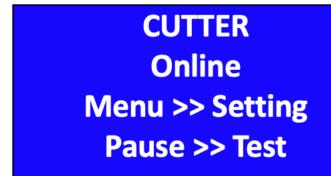
4.3.5: Press "Pause" when the cutter is not cutting, to cut a small test square. You can judge the cutting blade's length by this test. Press "Pause" during cutting to stop the plotter. Press "Pause" again to continue cutting.
