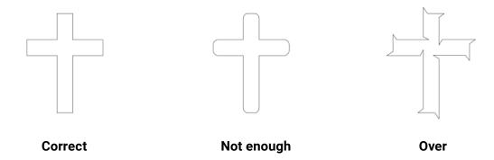
When you are using cutting software, we recommend you select the high precision output.
