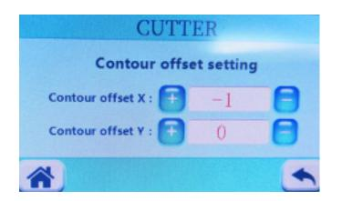
The cutter offset should be at 1 for 1mm.
