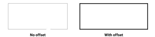
4.5.2 During cutting, if the right angles are not at right angles, please set the Sharp-angled compensation in the cutting software.
