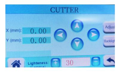
If the contour line shifts, change out the blade for a pen and move the carriage head into a blank space. Then, click "Backlight" first, then click "Adjust" and the cutter will automatically readjust itself. 4.3.5 Please DO NOT adjust the "XY scale", "Language" or "Burn In Test" on your cutter.
