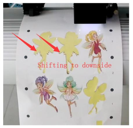
5. How to calibrate camera contour if it is shifting like the example below:
