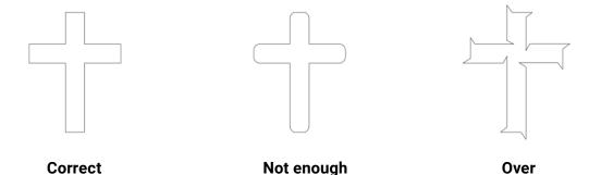
When you are using cutting software, we recommend you select the high precision output. For example, to cut vinyl, set offset to 0.25 with an overcut of 1-2. To cut 3M reflective film, set offset to 0.65 with an overcut of 0.65 and so on. Basically, you need to adjust the data and test before cutting your main design.
