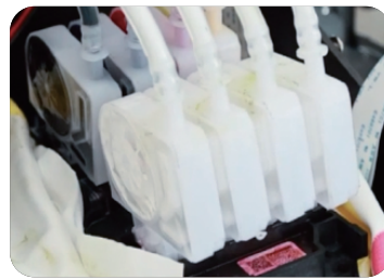
Arrangement of print head in the ink supply tube (K C M Y W W W)
