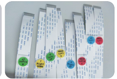
Data cable: 14-core flat cables connecting the print head to the headboard, with 4 cables required per print head.
