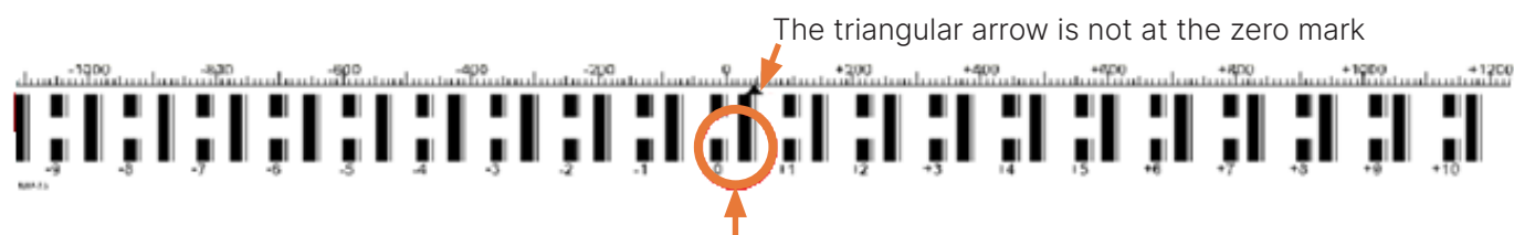
The two black sections on the left and right do not overlap each other Nozzle horizontal spacing alignment state figure 2
