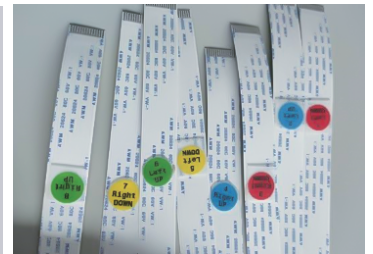
Data Cable: 14-core flat cable connecting the printhead and headboard; each printhead requires 4 cables
